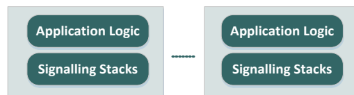
Non-Distributed Architecture: Signalling and Application modules share the same process. Scaling requires separate signalling modules and licenses.
